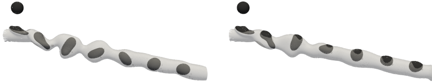
Figure 1: Exemplary droplet-jet interaction of a fully (left) and partially wetting (right) liquid combination.
